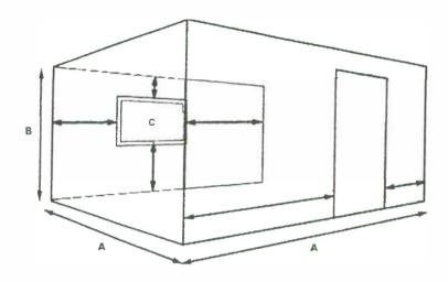
The first step is to measure all the walls from corner to corner (A), marking on your plan anything that projects into the room or recesses out. Measure the ceiling height (B) and clearly mark any changes in that height.
